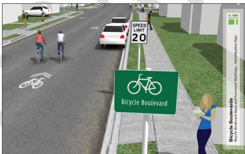
Figure 1 – NACTO Urban Bikeway Design Guide Bicycle Boulevard: Signs and Pavement Markings Illustration
