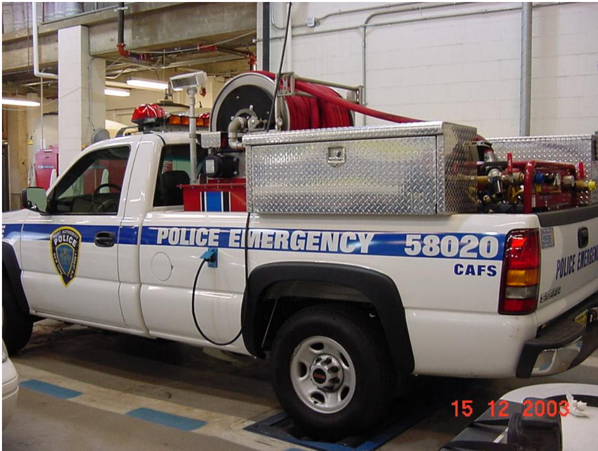
Figure 5. QRV Deployed as Frontline Fire Suppression Vehicle
