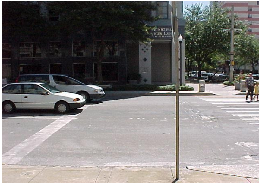
Figure 1-8: A picture of an advance stop bar at a traffic signal
